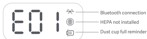
Brush roller overload protection
